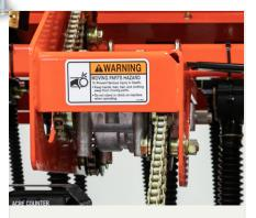
4-Speed gearbox provides increased accuracy and flexibility of the metering system by giving the operator more choices for drive speed.
