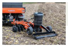
The rear roller gently presses seed into the ground for good seed-to-soil contact. It pivots for transport and storage without taking the spreader off the unit (shown below).
