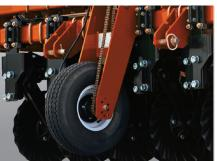
The ground drive system automatically disengages when lifted, simplifying the unit and enhancing its reliability.
