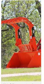
Wide 84" jaw opening allows operator to grasp large loads.
