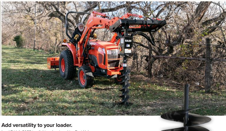
Land Pride's SA20 is a lighter planetary drive Post Hole Digger ideal for land owners, landscapers, hobby farmers, or contractors. The SA20 digs holes from 9" to 36" in diameter and up to 48" deep or deeper with available auger extensions. With a variety of augers available - 7 double flight augers from 9" to 36" and 3 tree augers in 24", 30", and 36" sizes, the SA20 is a versatile and dependable tool.
