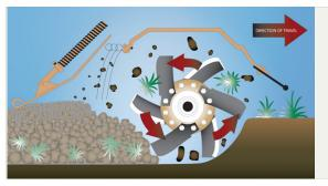
The reverse rotation of the tiller tines forces the tiller in the ground, preventing "walking" on hard ground. Once it's in, it stays put!
